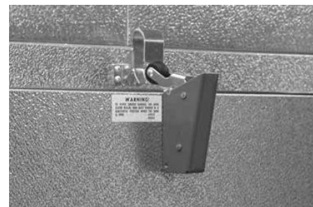
Roller Too High
